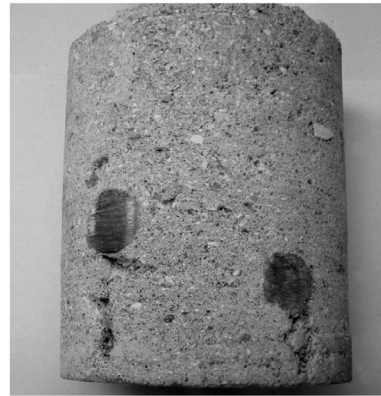
Dry-mix shotcrete, intersection #4 bars, linear defect from bar extending to back of panel. No interconnection detected or void against panel.
