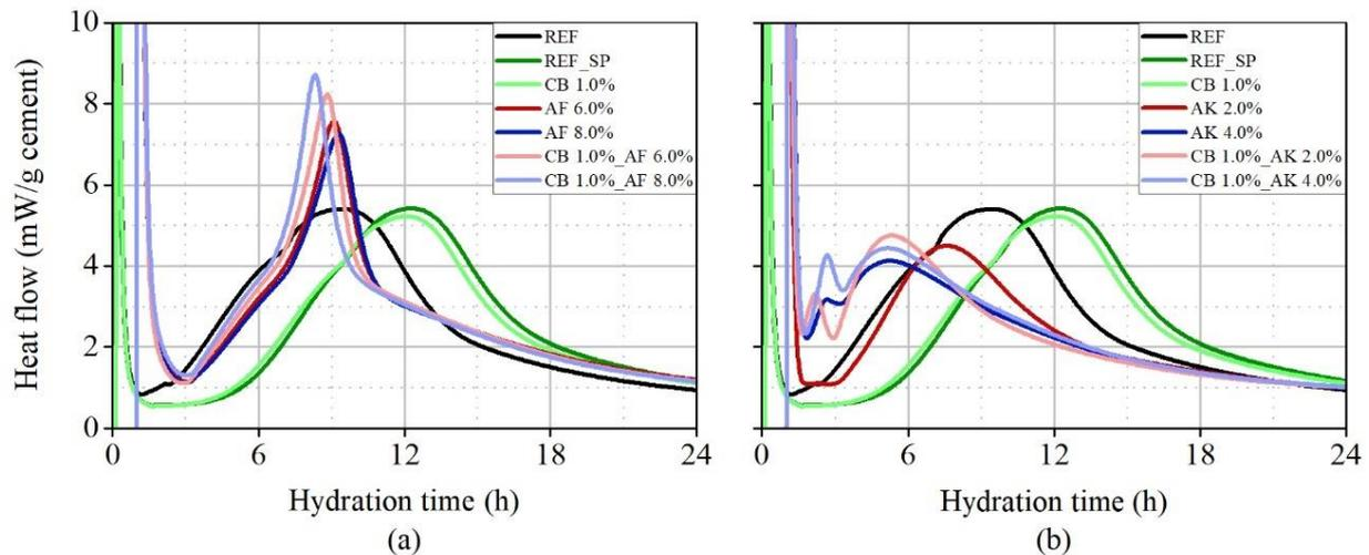
Figure 1: Heat flow curves from 0 to 24 h obtained with cement pastes produced with accelerator AF (a) and accelerator AK (b)
