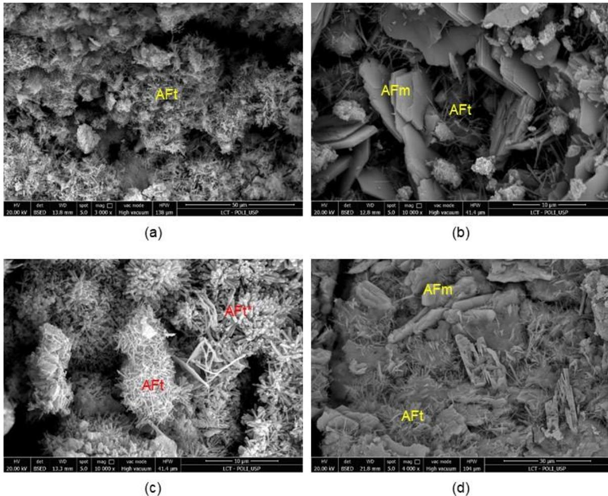
Figure 2: SEM images of cement pastes AF 8.0% (a) AK 4.0% (b), CB 1.0%\_AF 8.0% (c) and CB 1.0%\_AK 4.0% (d) 15 h after accelerator addition
