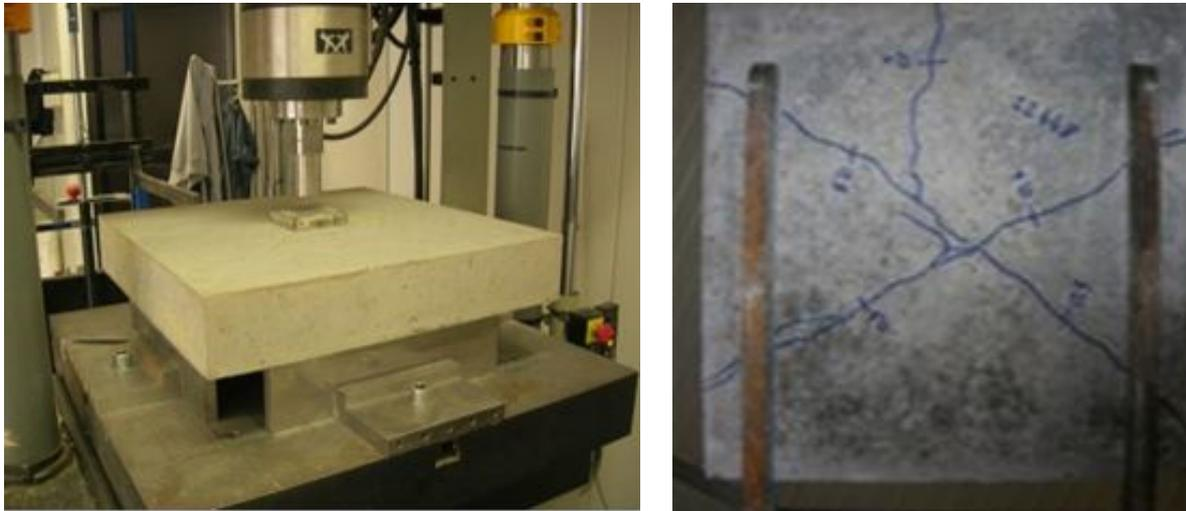
Figure 1 & 2: Square panel test according to EN 14488-5 (left) and crack pattern after 2 mm deflection (right)
