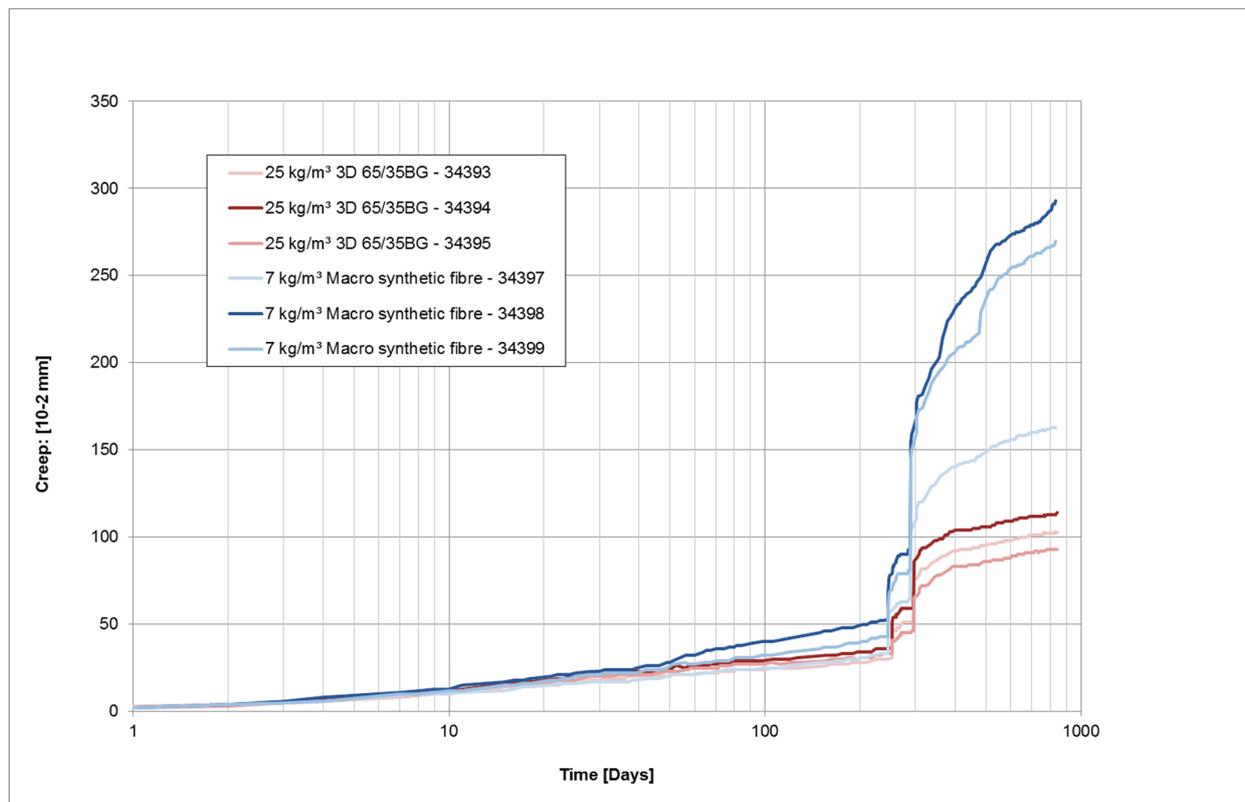
Figure 5: Creep behaviour of macro-synthetic and steel FRC
