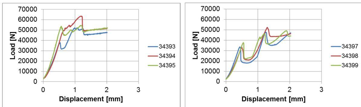
Figure 4: Initial test results for steel (left) and synthetic (right) FRC
